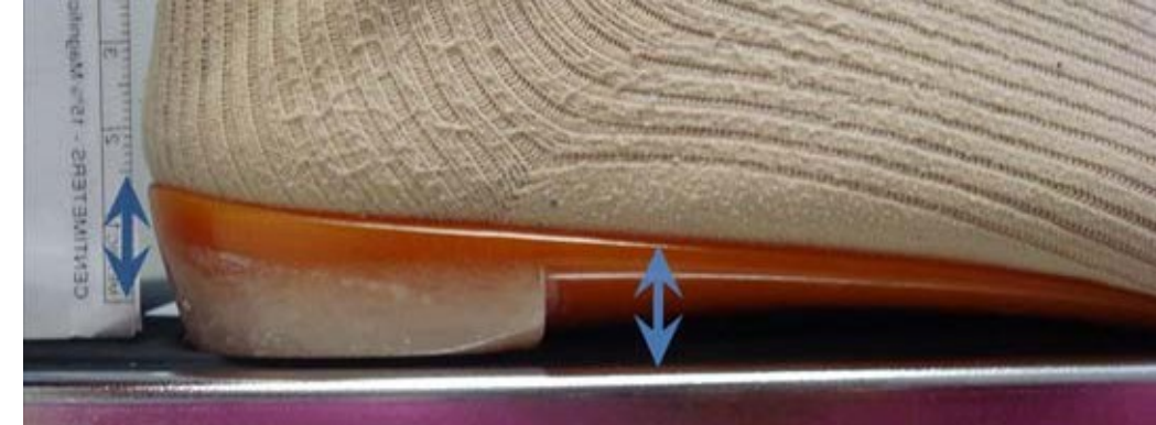
Figure 2: Acrylic Orthotic with subject standing on it. Lateral arch height is 4mm less, at 14mm.
